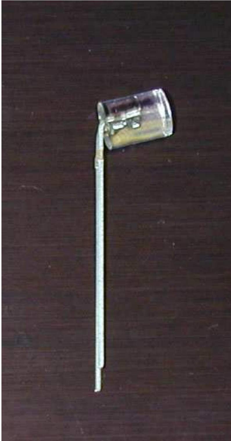
Figure 6 LED Lead Forming at 100 degrees (note short Cathode lead and lead bend close to LED body) ( note alternate LED part numbers may appear visually different than pictured above)
